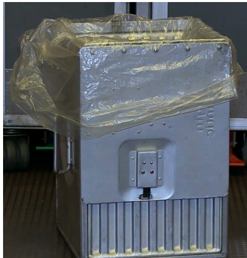
Figure 5.9 – A bar box made water-tight using a plastic bin liner
