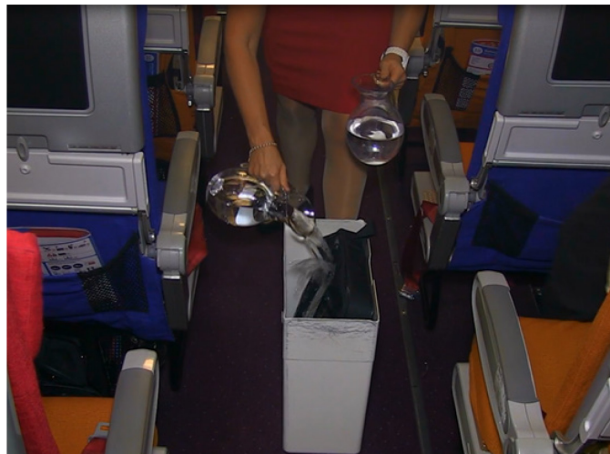
Figure 5.7 – A lap top computer in a bag being submerged in water in a toilet waste bin....
