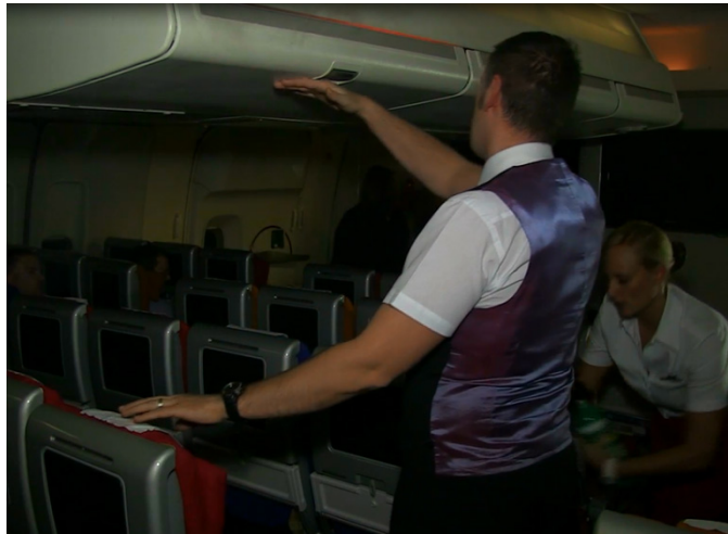
Figure 5.2 – Determining the location of a fire in an overhead locker
