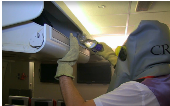
Figure 5.5 – Applying water to a lap top computer without removing it from an overhead locker
